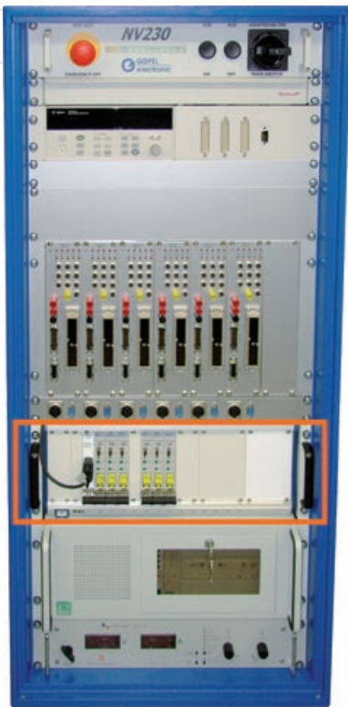
Figure 2. MOST PXI test system (six ways).
